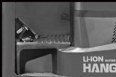
The pedal height can be adjusted electrically(Optional)
